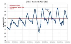
The cooler night ambient is used to store cool energy within the PCM passive cooling modules placed within the false ceiling area and this stored energy enables the day cooling loads / solar gains within the classroom is absorbed by PCM modules without using any mechanical cooling machinery.
